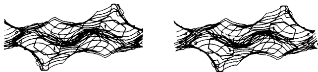
Figure 7. Stereoscopic drawing of the cavity enclosing the trans -stilbene (centered on (0, \frac{1}{2}, 0) ) in the channel parallel to the a axis. The contours of the volume accessible to stilbene atoms are drawn in sections separated by 0.40 \text{ \AA} and parallel to the (a,b) plane; they are viewed normal to the (a,b) plane and are included in a parallelepiped defined by -0.79 \leq x \leq 0.69 , 0.25 \leq y \leq 0.75 , -0.12 \leq z \leq 0.12 . A point is considered as accessible to stilbene atoms if its distance to the van der Waals envelope of TOT is larger than 1.5 \text{ \AA} .
